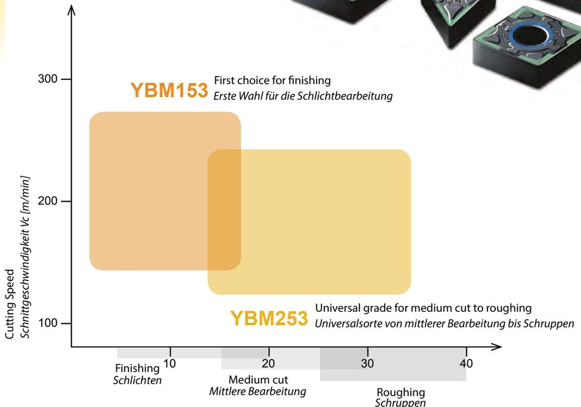
**Solution for stainless steel and materials which are hard to machine**
